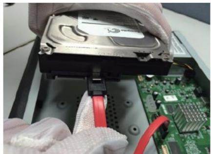
3. Connect one end of the HDD power cable to the interface of the NVR mother board and the other end to the HDD.
